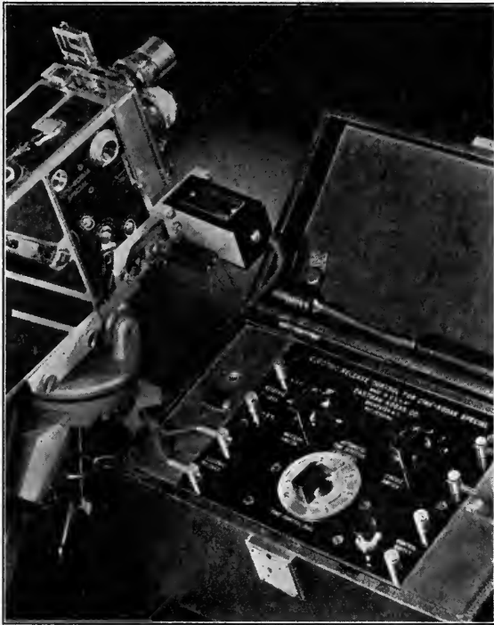
FIG. 1. The Electric Release Control for the Cine-Kodak Special, consisting of the Electric Release, which is mounted on the camera, and the Electric Release Control box, which supplies the necessary impulses to control the camera action.
